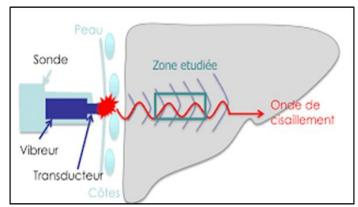
Figure 1: Positioning of the probe and volume of parenchyma explored (Echosens image)
