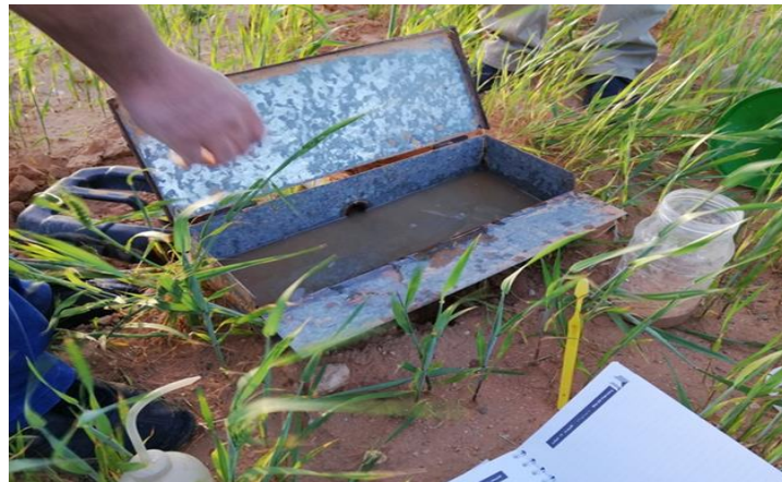
Fig 4: Gerlesh trough to collect runoff water and sediment soil
