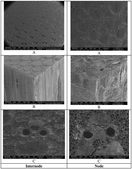
Fig-2: SEM images of the vascular bundles at internodes and nodes of the G. scortechinii
