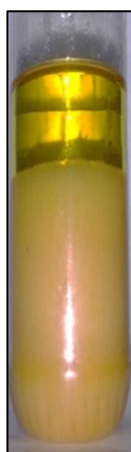
Fig-2: Biofuel oil is at the up layer of the flask in translucent yellow color while the bottom layer is the glycerol layer (The experience was done at the Faculty of Engineering at Port Said University)
