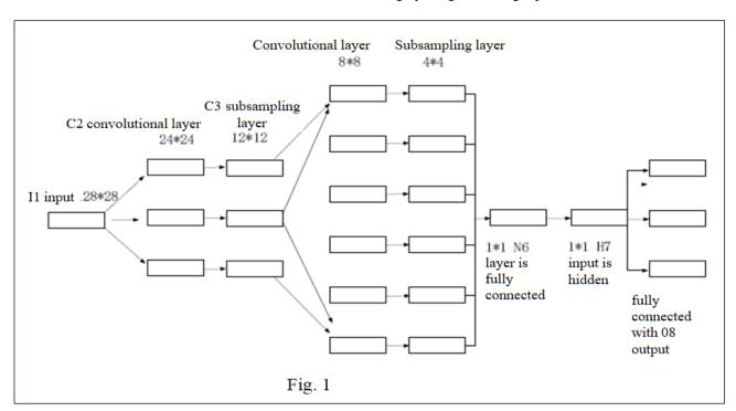
Recognizing human gestures by using the convolutional neural network specifically as follows.
