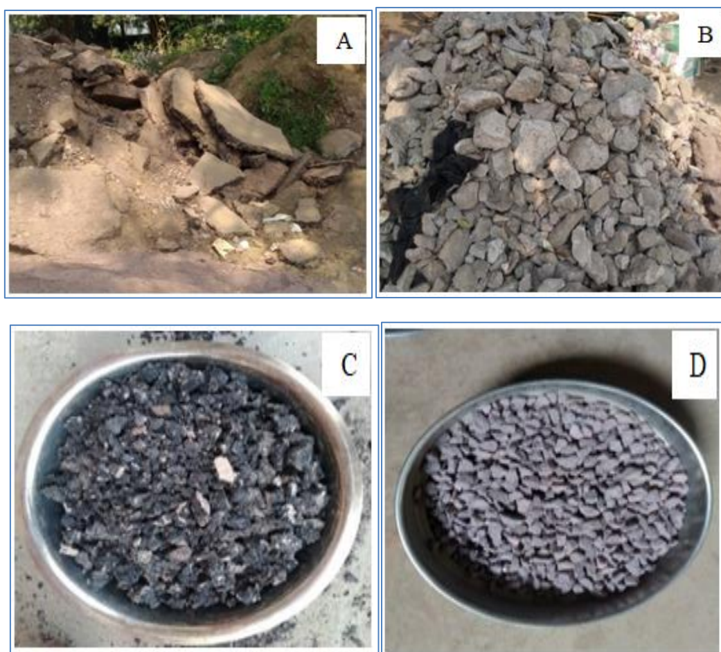
Figure 1: Recycled aggregates, (A, B) road demolition, (C) build demolition, (D) prepared sample
