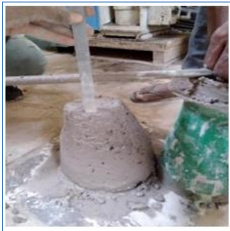
Figure 3: Slump test on concrete study
