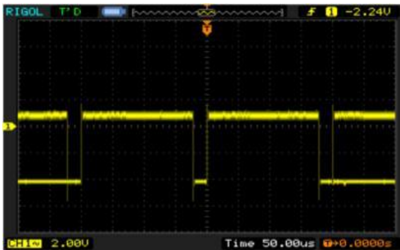
Figure 15: Bulk charging wave shape
