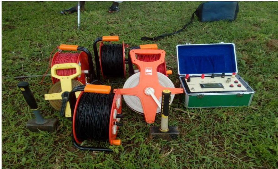
Plate-1: Picture showing the Petrozenith Terrameter and some other instrument that was used for the survey
