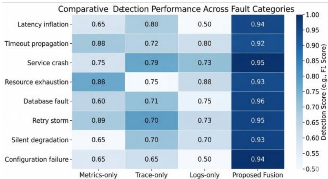
Figure 3: Detection performance across fault categories for baseline methods and the proposed fusion model
