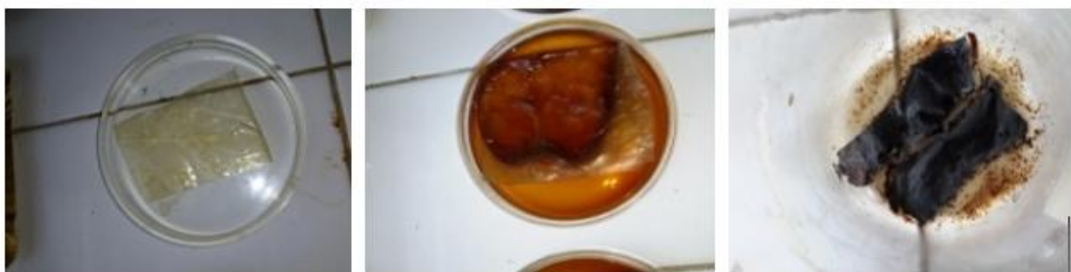
Fig-10. Plastic before being given EM4 (left), after being given EM4 (middle), and after 35 days of degeneration (right)
