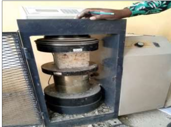
Figure 3: Compressive Strength Testing of NPFRC Sample
