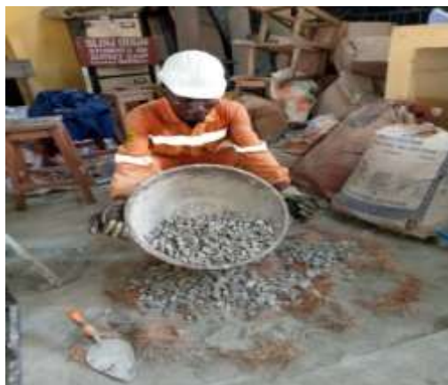
a) Mixing of fibre with cement and aggregates
