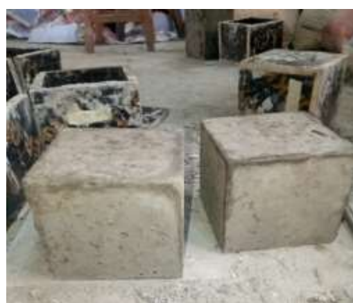
d) 24 hours concrete cube specimen after Demolding
