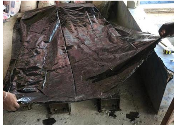
Fig-1: Covering of the concrete cubes and beams produced
