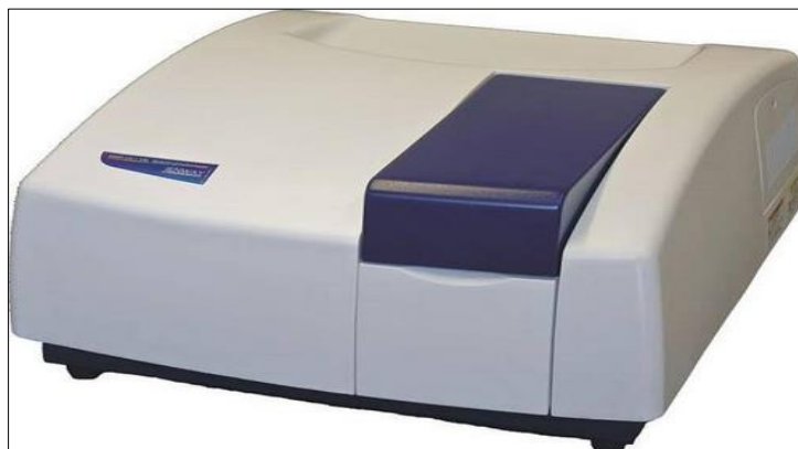
Fig. 16: Double beam spectrophotometer (Ramzy, 2021)
