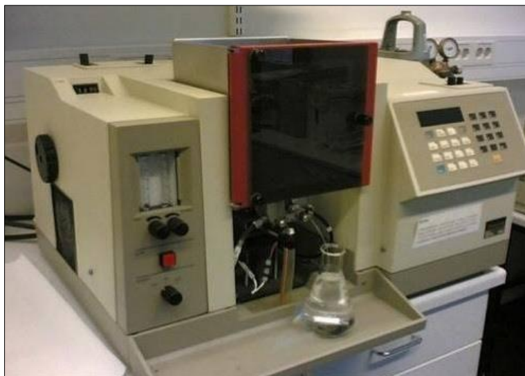
Fig. 22: Atomic absorption spectrophotometer (Ramzy, 2021).
