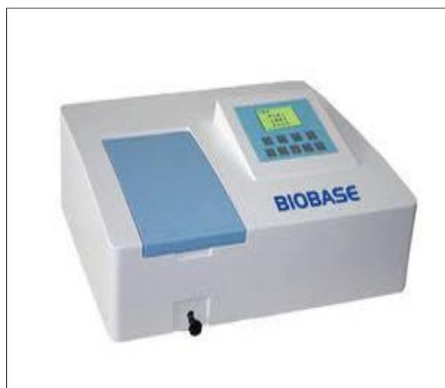
Fig. 15: Single beam spectrophotometer (Ramzy, 2021)
