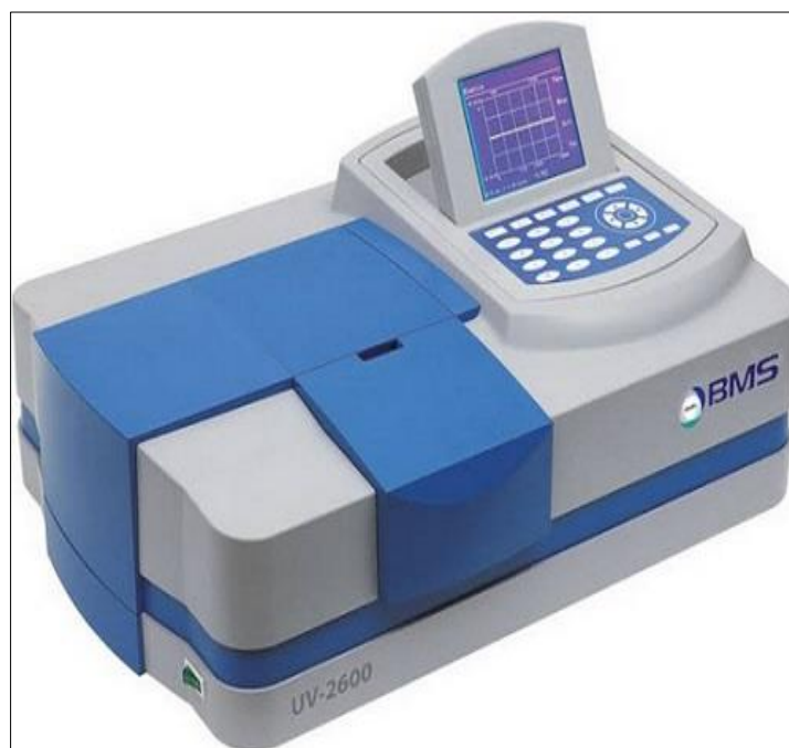
Fig. 17: Split beam spectrophotometer (Ramzy, 2021)
