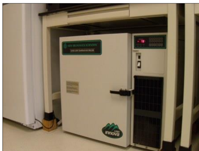
Fig. 50: Ultra-Low Temperature Freezer (CLST, 2020)
