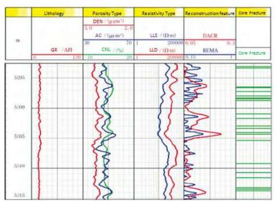
Fig-5: Identification of fractures using reconstructed log curves
