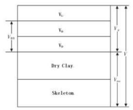
Fig-1: Geological model of double pore structure
